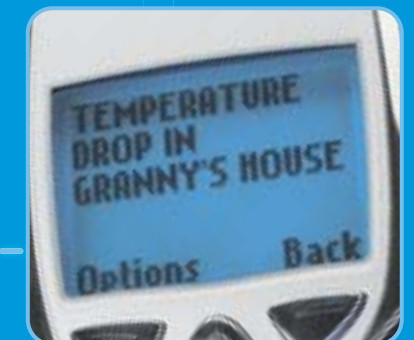
Users can define the message that each of four separate triggers send to telephones.
